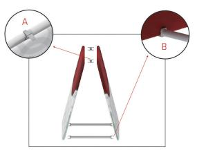
4. Connect the two frames together from the top using two plastic clamps (A). Then connect the fames from the bottom using two aluminum poles (B).
