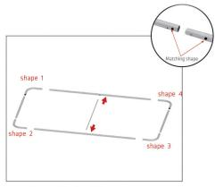
1. Assemble the different sections of the frame by matching the shapes on the poles.
